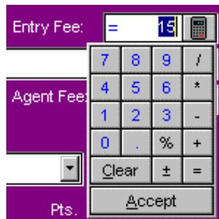
Typing in numbers and using the +, -, \*, / keys, you can use the keypad like a calculator. Click the Accept button or press the Enter key to close the calculator and save the calculation. Press the ESC key or click the Clear button to close the calculator without saving any result.
